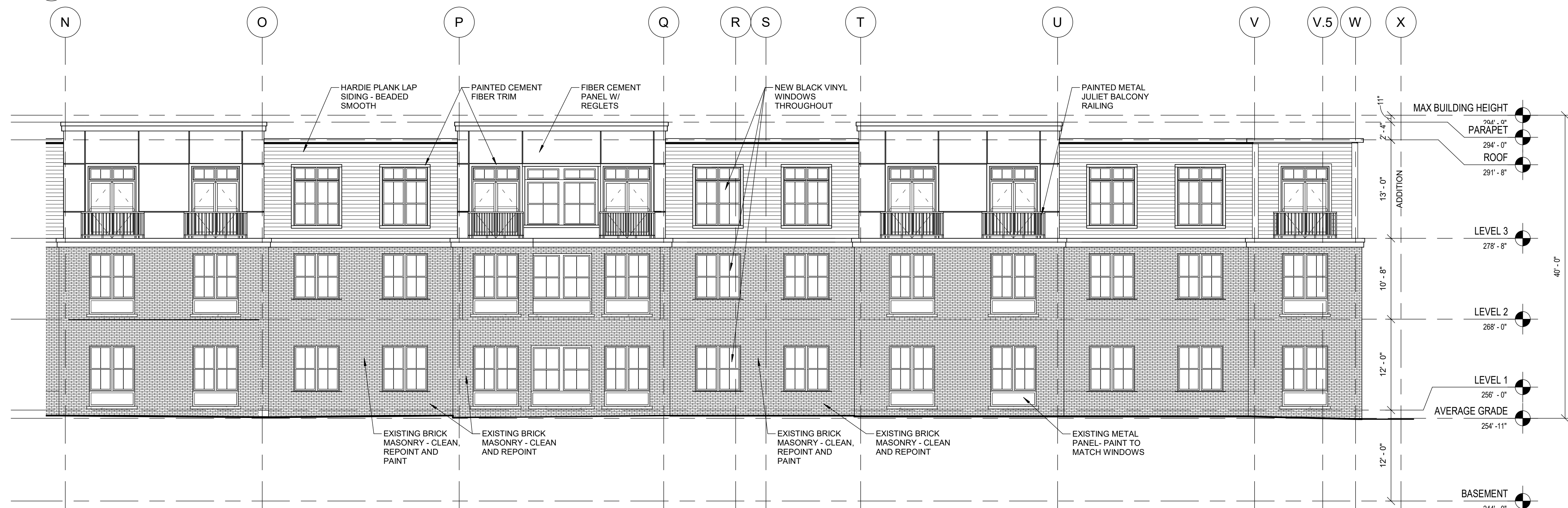
11 GOULD STREET ELEVATION - B Scale: 1/8" = 1'-0"
